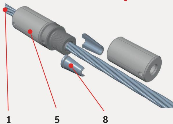
**Fig.12.2** Mono-Coupler Axonometric View
