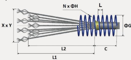
**Fixed Bulb Anchorage Side View**
