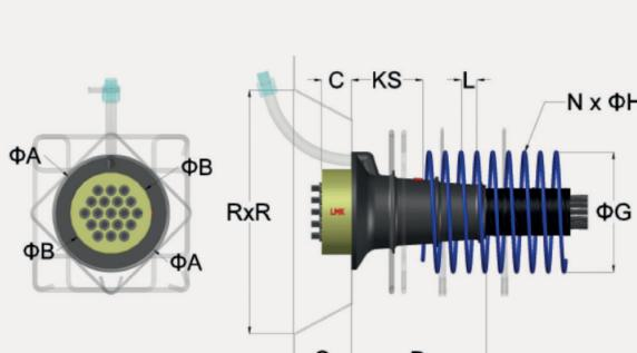
Stressing Anchorage Front & Side View
