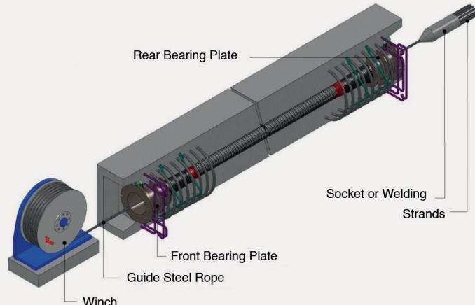
**Fig.4 Pulling Method Configuration**
