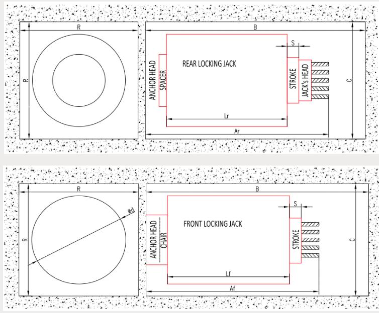
**Fig.17 Required Jacks Clearance**
