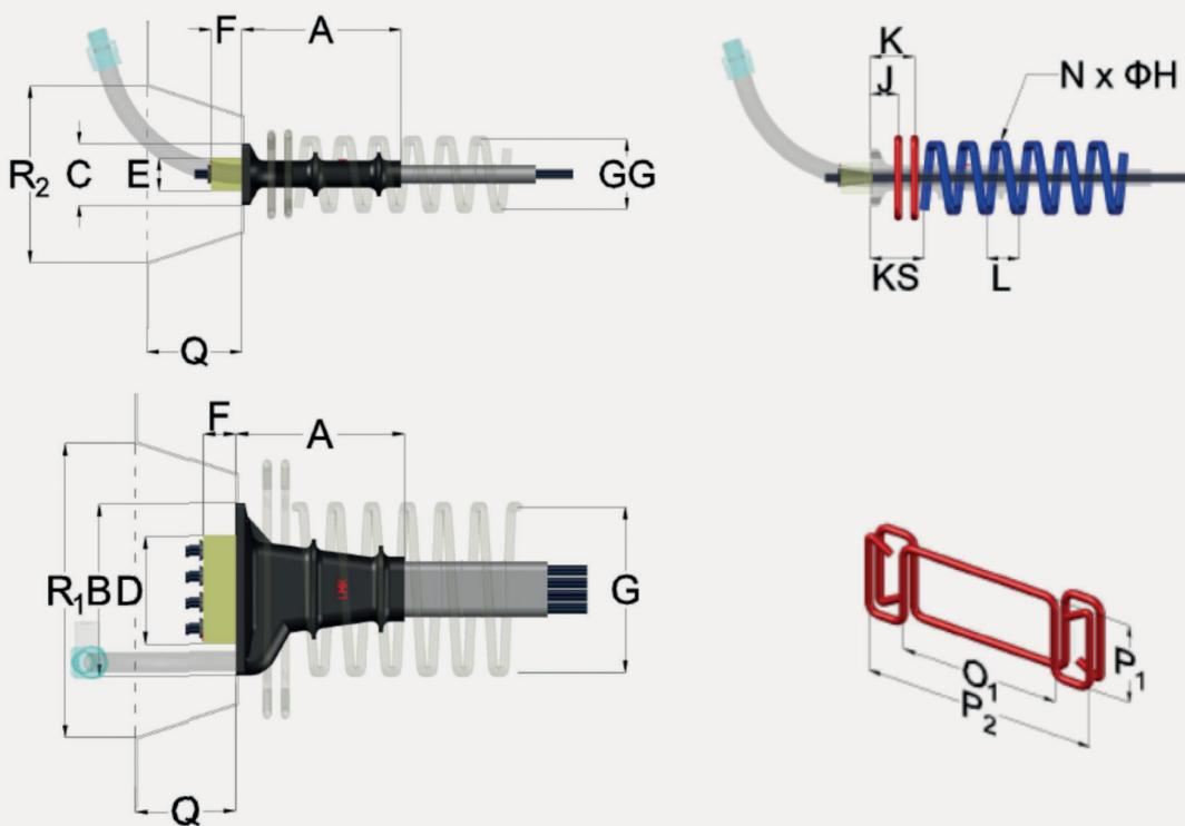
Stressing Anchorage Side &amp; Plan View
