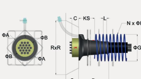
Stressing Anchorage Front & Side View
