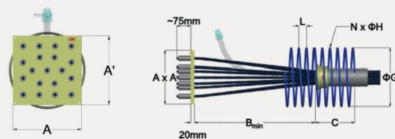
Fixed Swaged Anchorage Front & Side View
