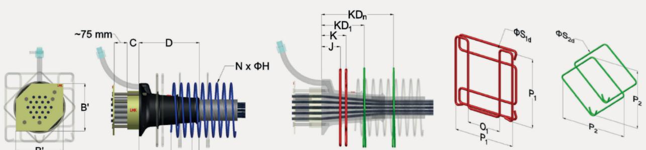
Stressing Anchorage Front & Side View
