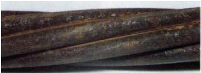
BEFORE CLEANING – ACCEPTABLE BUT CLOSE TO LIMIT- AFTER CLEANING
