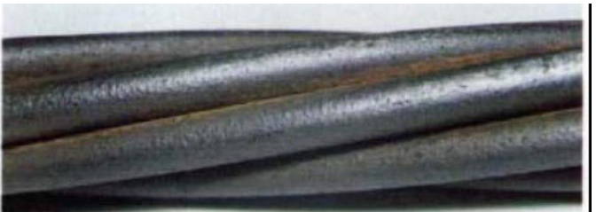
BEFORE CLEANING – ACCEPTABLE BUT CLOSE TO LIMIT- AFTER CLEANING
