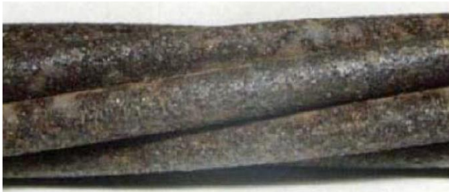
BEFORE CLEANING – REJECTED- AFTER CLEANING
